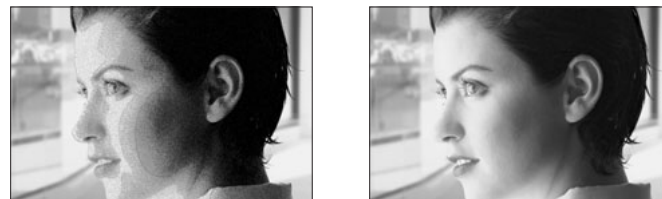
Conventional Plasma Display Panel False contours lower the picture quality
